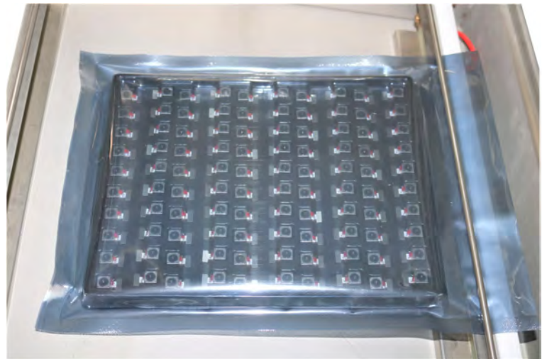
Vacuum the Anti-Static Bag
